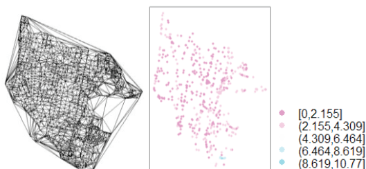
Fig. 2. (a) Delaunay Triangulation; (b) Depth estimation map for wells not measured by TIN
