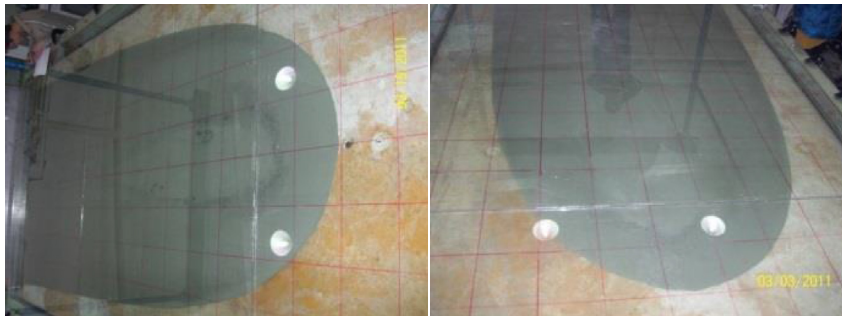
Fig. 3. Stabilized diffusion pattern of cement grout.
