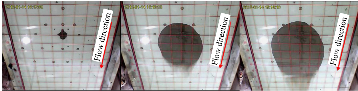
(a) Transient diffusion patterns of fast curing grout under dynamic water condition.
