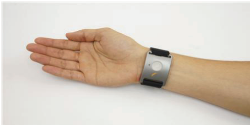
Fig. 3. Skin conductance sensor indicating objective arousal
