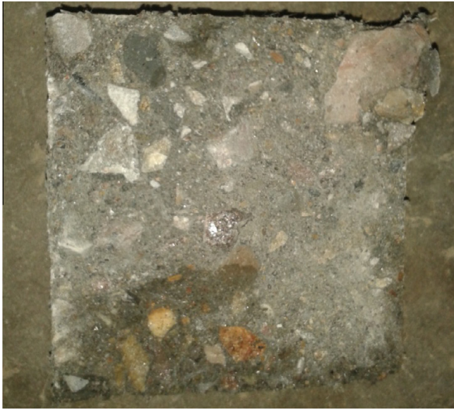
Figure 10. Water front penetration depth on splitted cube after permeability test.
