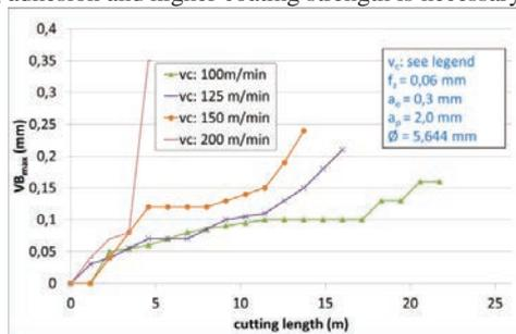
Fig. 10. Wear as a function of cutting length at milling of Inconel 718 with different cutting speeds  $v_c$ .
