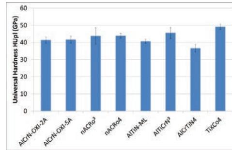
Fig. 7. Coating hardness of the deposited coating systems
