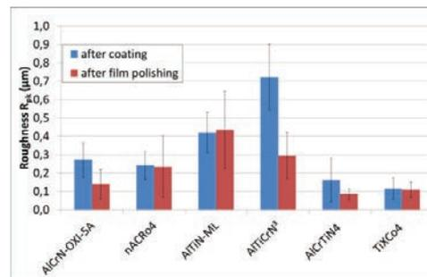
Fig. 8. Roughness R<sub>pk</sub> on cutting edges pre and after film polishing for different coating systems
