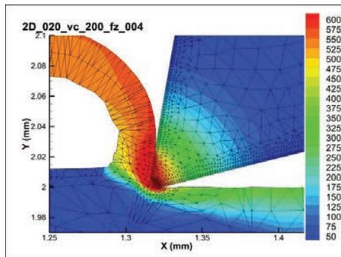
Fig. 3. Typical temperature field, used parameters:  $f_z=0,04$  mm,  $v_c=200$  m/min,  $a_e=0,3$  mm,  $a_p=2$  mm, cutting angle=10°, clearance angle 14°
