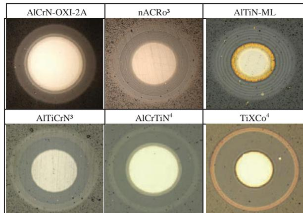
Fig. 6. Film structures of selected coating systems
