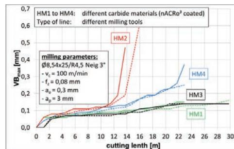
Fig. 5. Milling of Inconel 718 with different carbide materials
