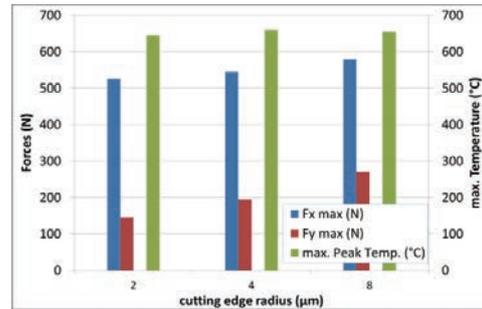
Fig. 4. Cutting forces and cutting temperatures as a function of the cutting edge radius of the milling tools
