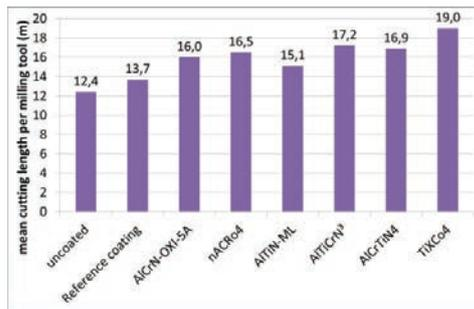
Fig. 9. Mean cutting length per tool for a wear  $VB_{max}$  of 0.2 mm
