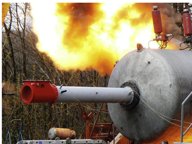
Figure 5 A back-flap installed on a pipe (RSBP, internal doc).
