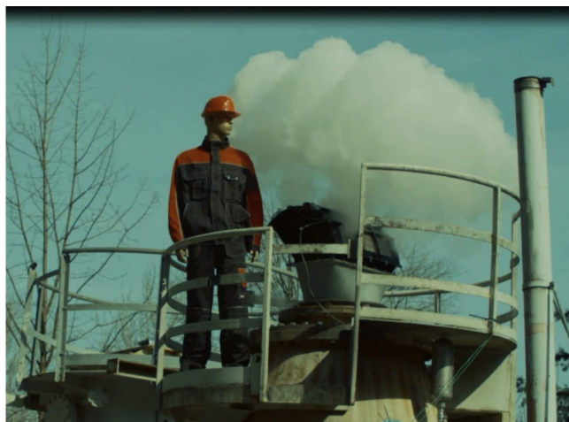
Figure 4 Flameless explosion relief on a testing vessel (RSBP, internal doc).
