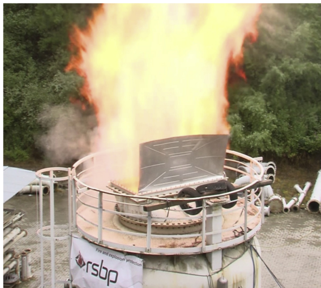
Figure 3 Explosion relief on a testing vessel (RSBP, internal doc).
