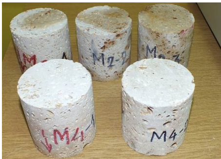
Fig. 10. Stone cylinders prepared for testing of compressive strength
