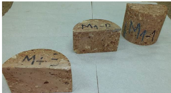
Fig. 11. Brick's semi-cylinders prepared for testing the bulk density and water absorption
