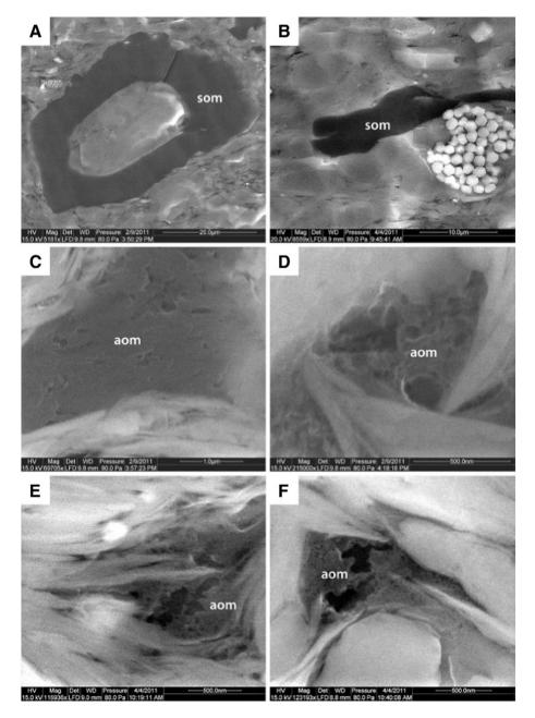
Fig. 28. Secondary electron images of gas-mature (>2.0% R<sub>o</sub>) Marcellus Formation organic matter. A and B Structured organic matter (som). C–F. Amorphous organic matter (aom). From Schieber (2013).
