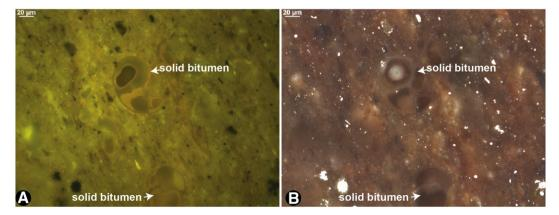
Fig. 22. Photomicrographs of organic matter in organic-rich (~6 wt.% TOC) immature (~0.25% BR<sub>o</sub>) Monterey marl outcrop sample, Santa Barbara County, California. A. Fluorescence, oil immersion. B. Same field as A in incident white light, oil immersion.
