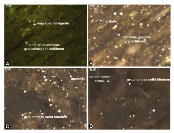
**Fig. 19**. Photomicrographs (oil immersion) of the Niobrara Formation. A–B. Immature (0.26% BR<sub>o</sub>) organic-rich (6.84 wt.% TOC) Niobrara marl from 591 ft. (180 m) in the Amoco No. 1 Rebecca K. Bounds well, Greeley County, western Kansas. A. Fluorescence illumination. B. Same field as A in incident white light. C–D. Peak oil window (~1.02% BR<sub>o</sub>) organic-rich (2.75% TOC) Niobrara marl (Niobrara B) from outcrops at the Cemex quarry near Lyons, Colorado, incident white light.
