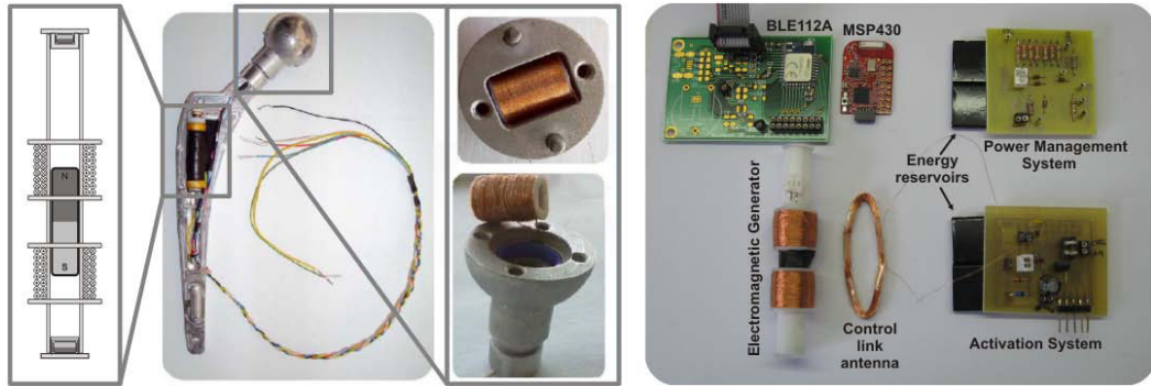
Fig. 2 Micro-power generators developed to work alongside the multi-purpose power management system
