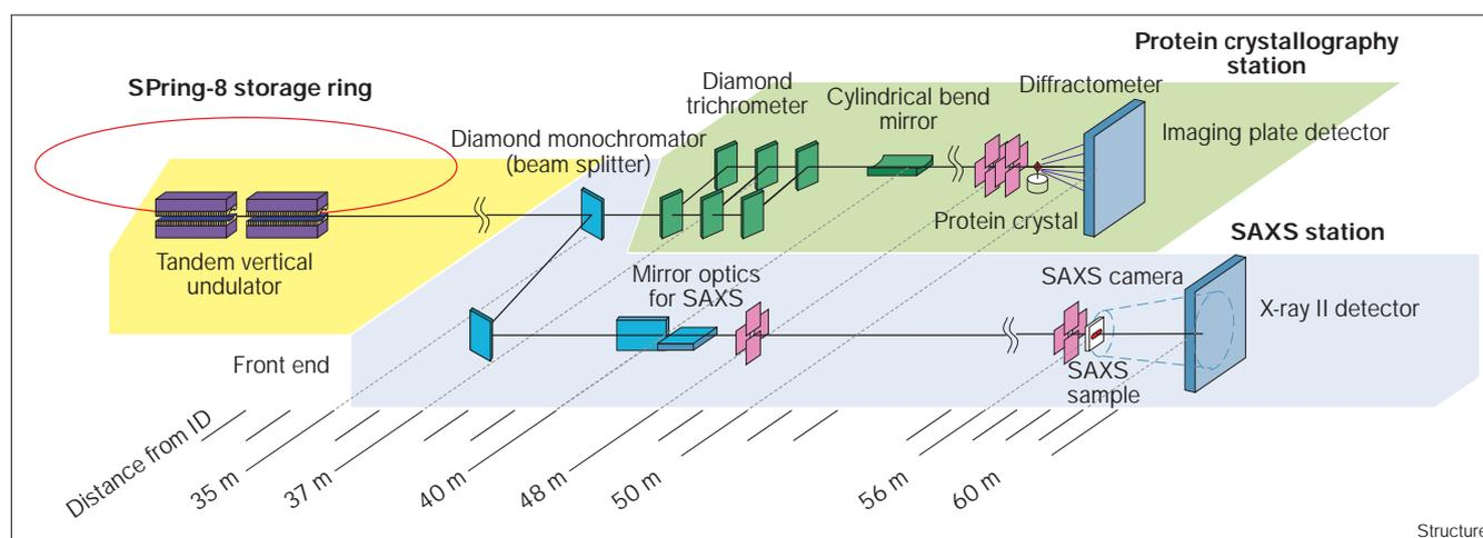
Outline of the RIKEN beamline I (BL45XU) for use in structural biology studies [4]. The main features of the beamline are illustrated; two tandem undulators and four sets of diamond crystal monochromators can be seen.
