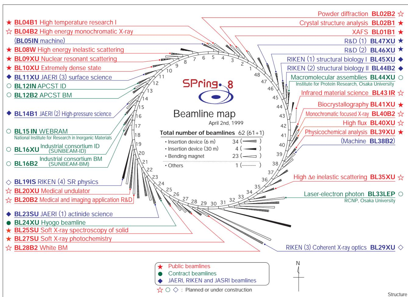
The beamlines at SPring-8. Beamline BL38B1 is not shown in the figure as the construction plan for this beamline has not officially been approved.
