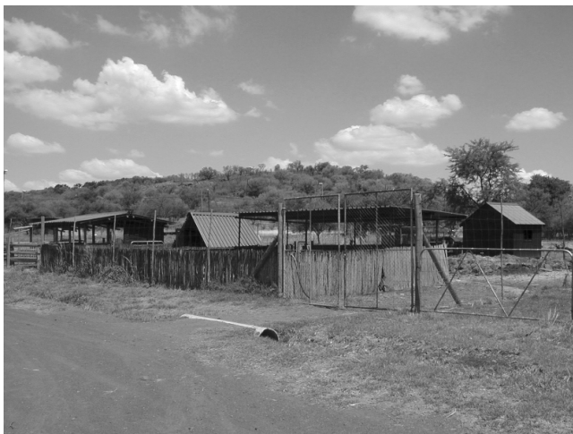
Figure 2: The kraal for sheep and/or goats, a poultry enclosure and the dairy unit are built with inexpensive materials such as poplar branches and reeds
