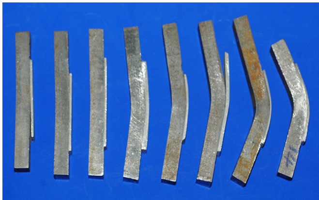
Fig. 6. Samples after face bend test.
