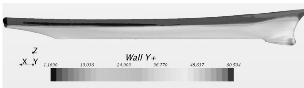
Fig. 7 Distribution of y^+ for fine mesh on hull.
