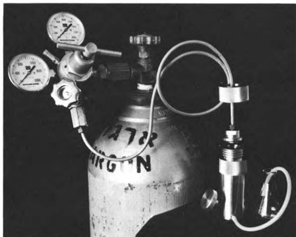
Fig. 1. A photograph of the Yeda Press. The instrument is shown connected to the pressure tank as in actual operation, but not closed, to illustrate the component parts.
