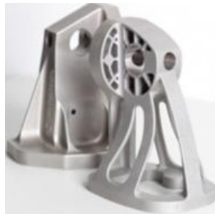
Fig. 1. Prototype of an optimized Airbus A380 bracket manufactured with AM (front) and investment casting (back) (EOS, 2014).
