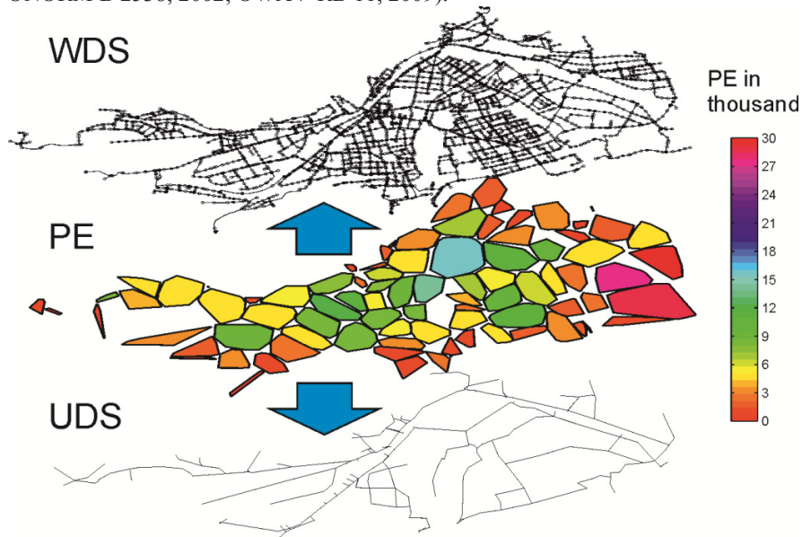
Fig. 1. UDS and WDS coupled via population (PE) for real world case study
