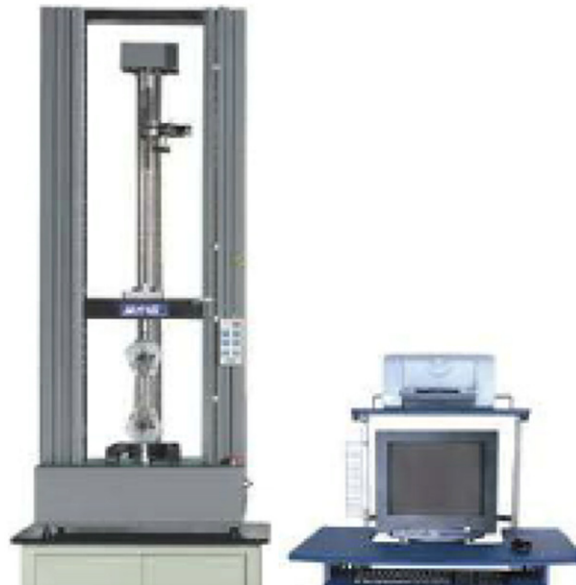
Fig. 3. CMT 6104 electrical universal material machine.
