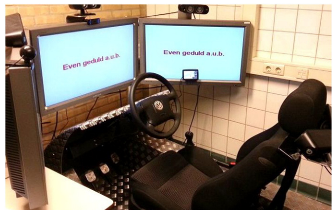
Fig. 1. The driving simulator, with the touch screen navigation system attached to the right hand screen.
