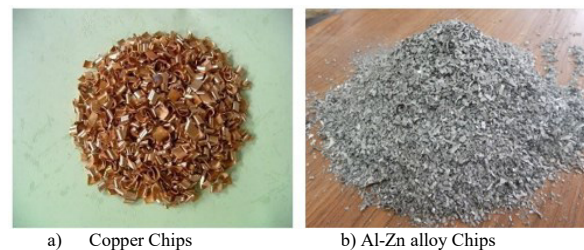
Fig. 3. Chips that generated from cutting operation as waste a) copper chips, and b) Al-Zn alloy chips.
