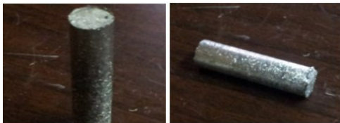
Fig. 6. Direct recycling shaft produced from chips of Al-Zn alloy with press pressure of 20 tons applied from one side.
