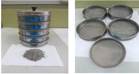
Fig. 4. Sieving tools used to measure size of chips.
