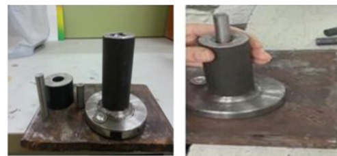
Fig. 2. Assemble of pressing mold (die and punch).
