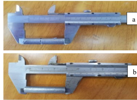
Fig. 7. Direct recycling shaft produced from chips of Al-Zn alloy with press pressure equal to a) 10 tons and b) 20 tons applied from two sides.
