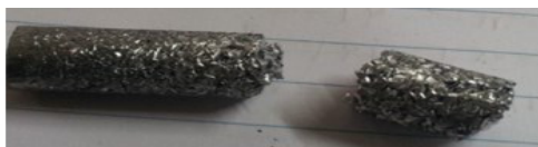
Fig. 5. Direct recycling shaft produced from chips of Al-Zn alloy with press pressure of 10 tons applied from one side
