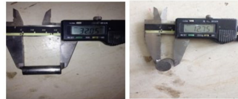
Fig. 8. Direct recycling shaft produced from chips of Al-Zn alloy with press pressure of 30 tons applied from two sides.
