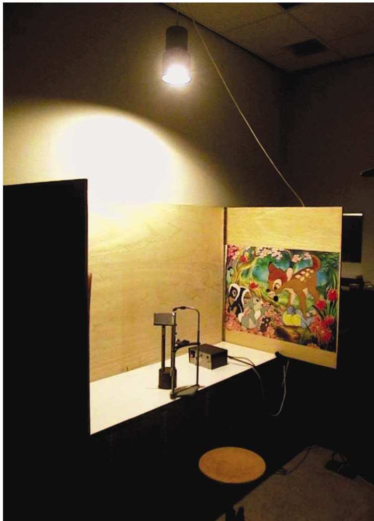
Fig. 1. Two screens with identical contrast- and colorful pictures were placed facing each other with two oblique-view mirrors halfway between them. Note the apparatus with a button for switching the two halogen lamps on for 300 ms.
