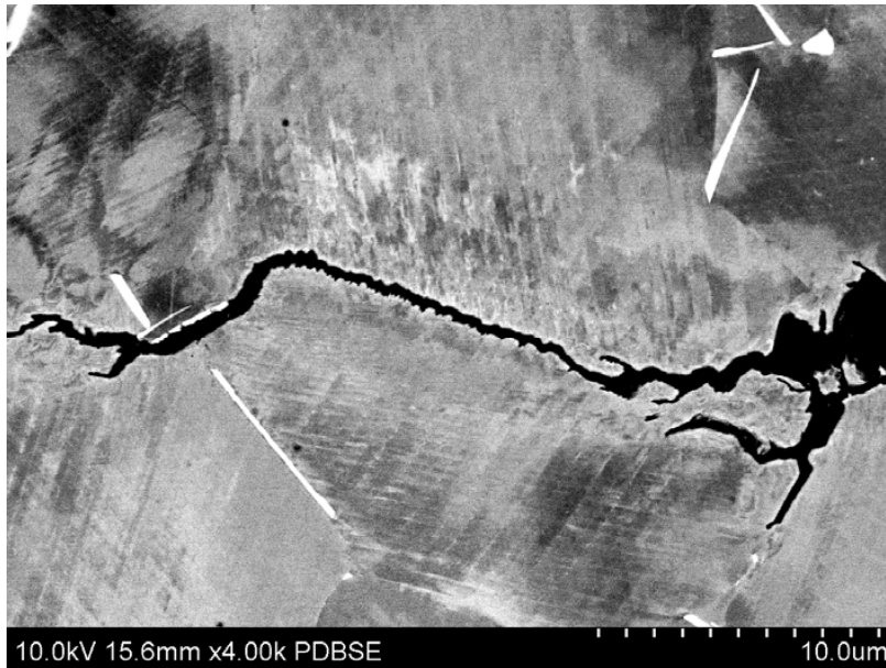
Fig. 8. Slip bands around the crack path of Baseline test at 650°C
