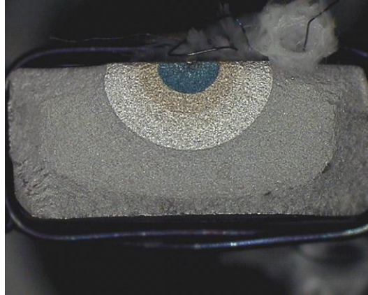
Fig. 2. Fracture surface of the calibration specimen with visible beach marks.
