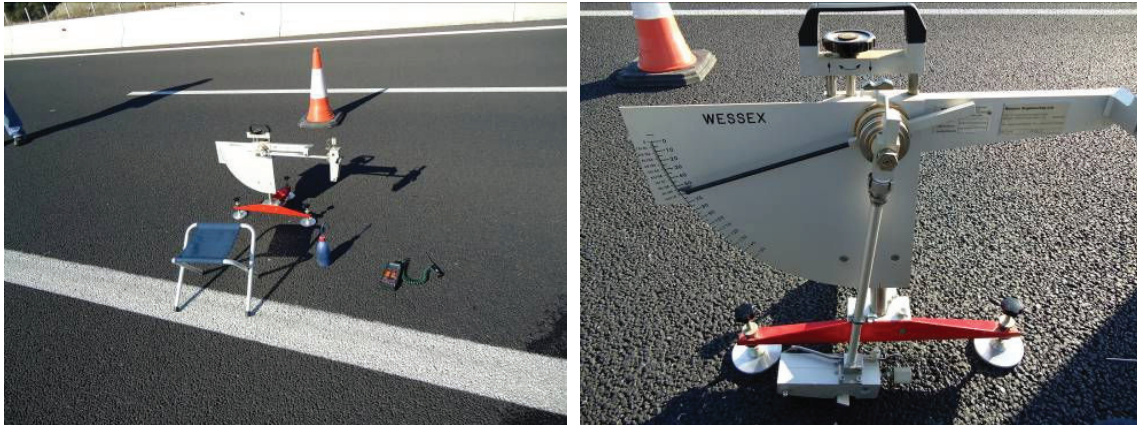
Fig. 2. Positioning and calibration of Skid resistance tester
