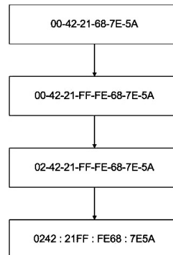
Fig. 2. EUI-64 interface identifier generation.
