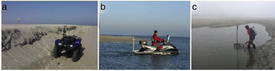
Fig. 5. Survey methods applied for the bed elevation measurements of the Sand Engine. a) Quad bike with RTK-GPS, b) survey jetski and c) RTK-GPS on a wheeled pole.
