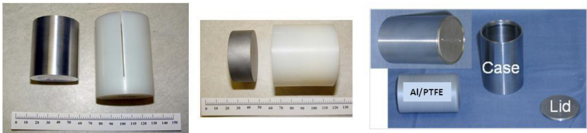
Fig. 1. Photographs of the aluminum, steel and aluminum cased Al/PTFE projectiles.
