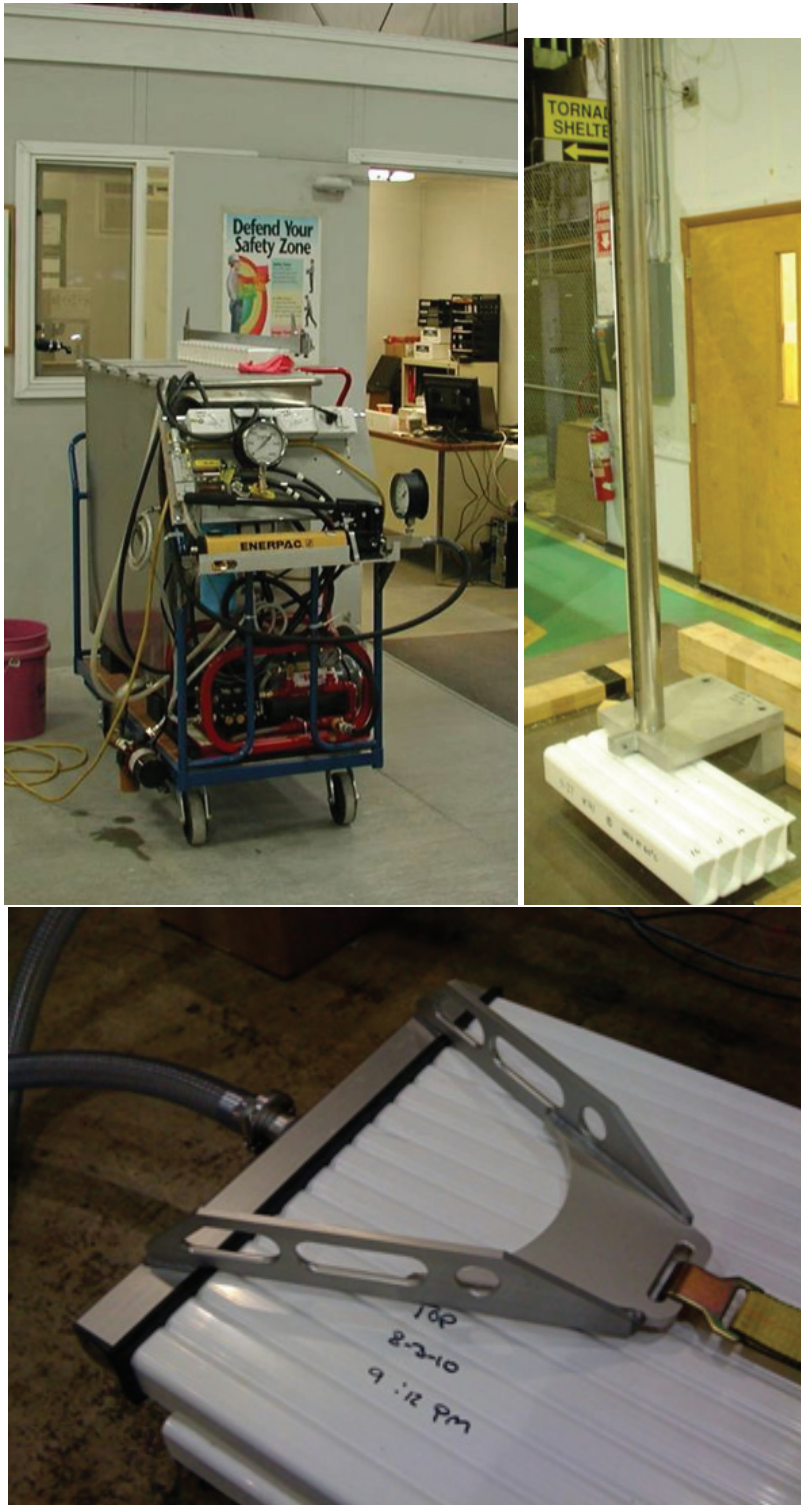
Fig. 5. Photographs of quality assurance tests of mechanical properties Pictures of the PVC QA tests, shown at the extrusion factory. In the top panel, the pressure test is on the left, the drop dart on the right. The vacuum test is shown on the bottom.
