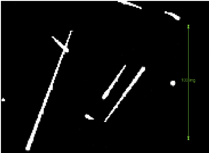
Fig. 1. Four muons tracks are clearly reconstructed on this image. There is a significant width different between the two ends of the track. The thicker end corresponds to the region of the track in the back of the CCD, with maximum diffusion. The thinner end corresponds to the front of the CCD. The smaller circular hits are diffusion-limited hits as expected for nuclear recoils. The line is 100 pixels long and was added to give a sense of scale.
