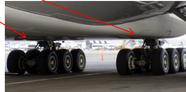
(b) detail of the belly gears with the two TDT gears
