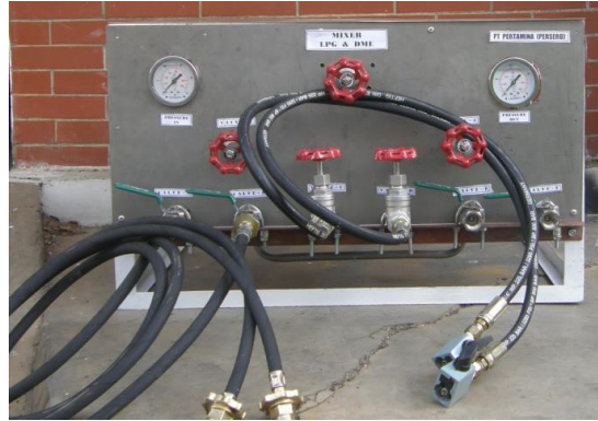
Fig. 2. LPG & DME blending unit (injector & manifold).
