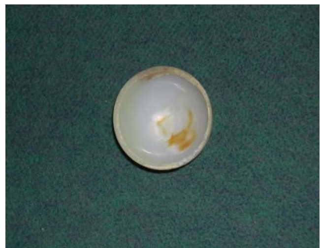
Figure 2 Low wear of the polyethylene component at 12 years.
