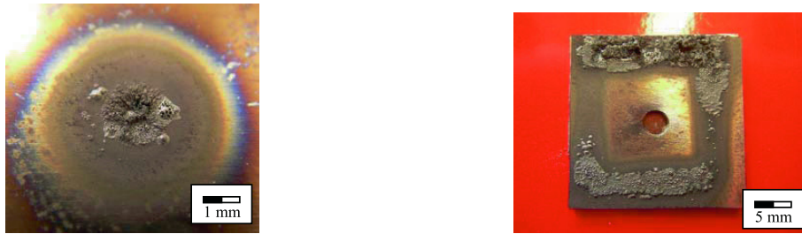
Fig. 5. Damaged upper metal sheet a) by spot joining, b) by contour joining
