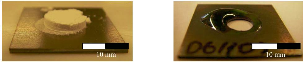
Fig. 10. Glass sealing material depot above the hole a) before, b) after the laser treatment
