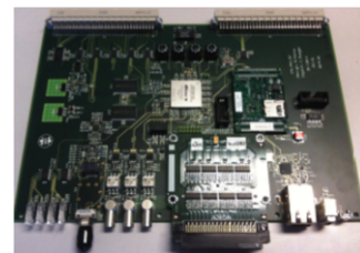
Figure 7: BCM1F VME Real-time histogram unit
