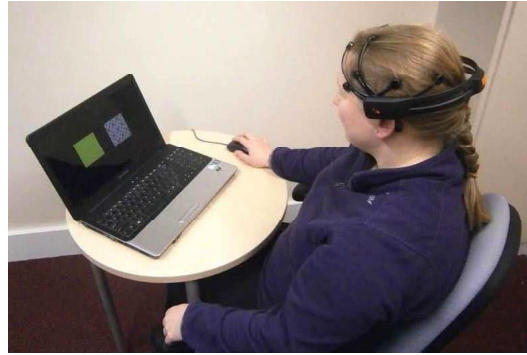
Fig. 1. Photograph showing the experimental setup using the Emotiv EPOC headset.
