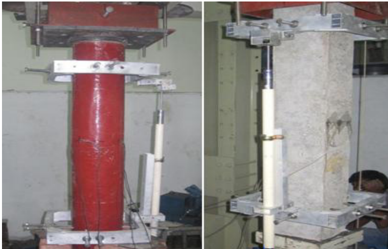
Fig.6. Laboratory test setup for RC columns
