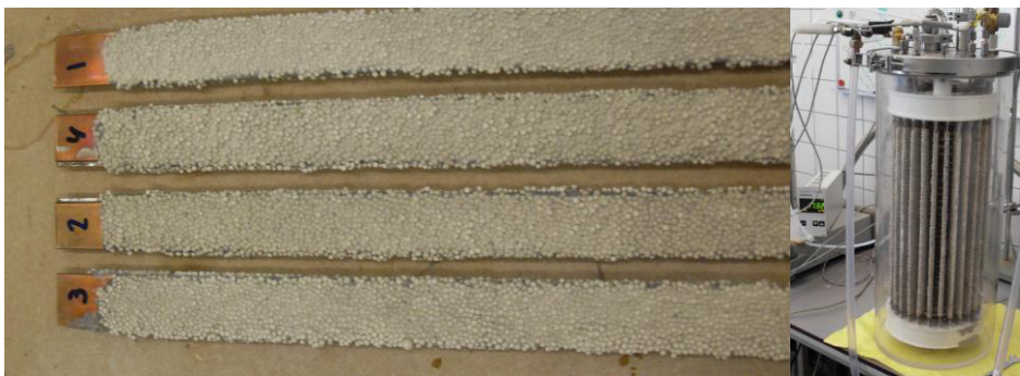
Fig. 4. (a) The real heat exchanger strips after theoretical optimization; (b) the built reactor with heat exchanger strips, evaporator/condenser, and measurement equipment.
