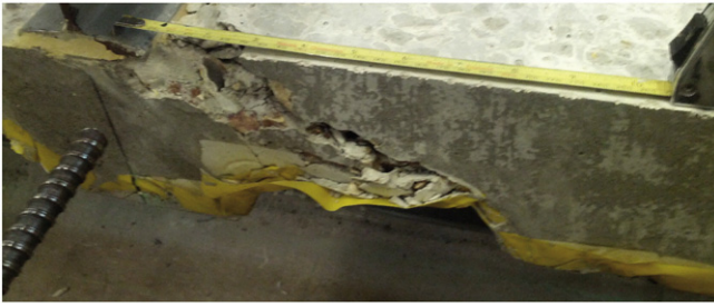
Fig. 8. Crack along a shear-plane, indicating compression failure of 2 m specimen.
