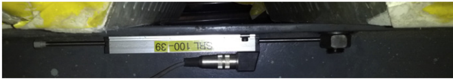
Fig. 4. Displacement gauge attached to the underside of beam top flange measuring relative slip of nut.
