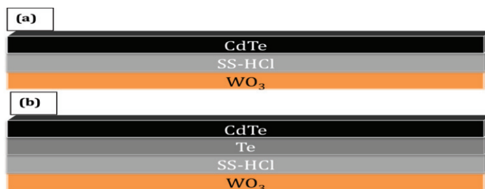
Figure 1. Cross-sectional schematic of hetero-type PEC electrodes with n-type tungsten oxide and p-type cadmium telluride on opposite sides of a stainless steel substrate.
