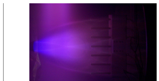
(a) Case 2-1, measure rake locating 250 mm away from nozzle exit plane
