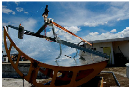
Fig 2. A prototype of CSP system at the RCEPM-LIPI [10].
