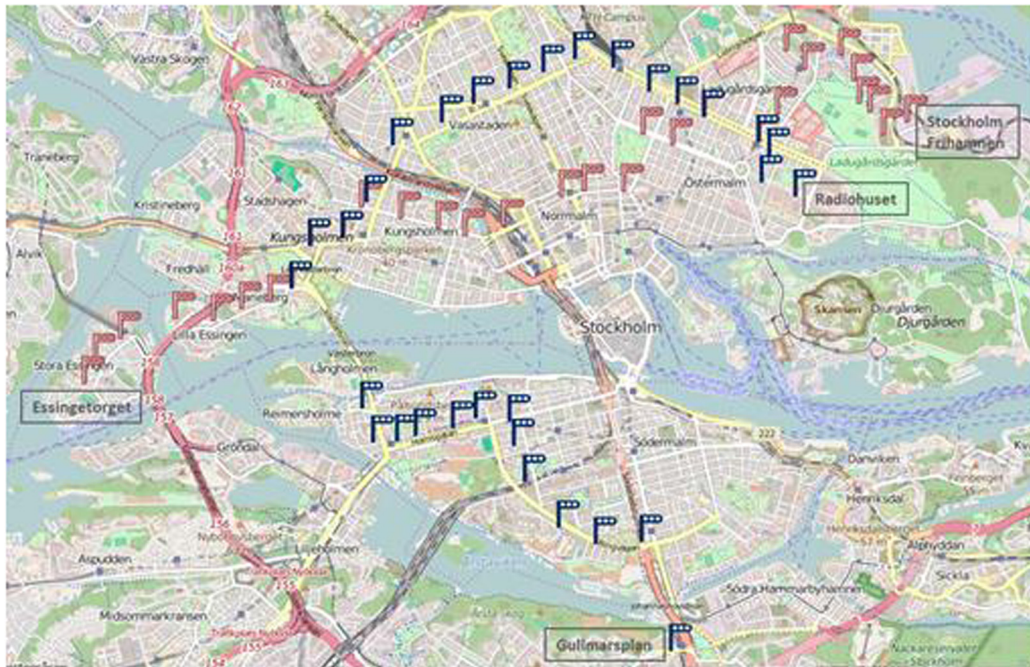
Fig. 2. Web-based visualization after querying bus services 1(bus stations in red), 4(bus stations in blue) from Sweden GTFS data with the use of Python GTFS library and OpenLayers.js (Fig. 3).
