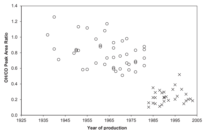
Fig. 8. FTIR results for animation cels showing the O–H to C=O peak area ratio versus year of production for cellulose diacetate (O) and cellulose triacetate (x) cels.
