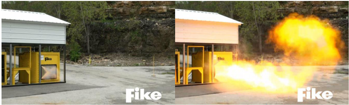
Fig. 3. Dust explosion venting test at Fike Remote Testing Facility: vent opening (left), and venting with flame release (right).
