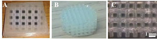
Fig.3. PLA scaffold fabrication process. A) Porous PLA printed bar with a zoom in (centre area) of top view (picture acquired with a stereomicroscope), B) Laser cut disc from A) and C) Laser cut disc surrounding edges.
