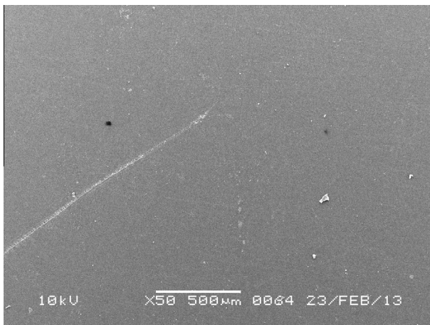
Figure 8 SEM image of visible light cured specimen after polishing using Universal Polishing Paste.
