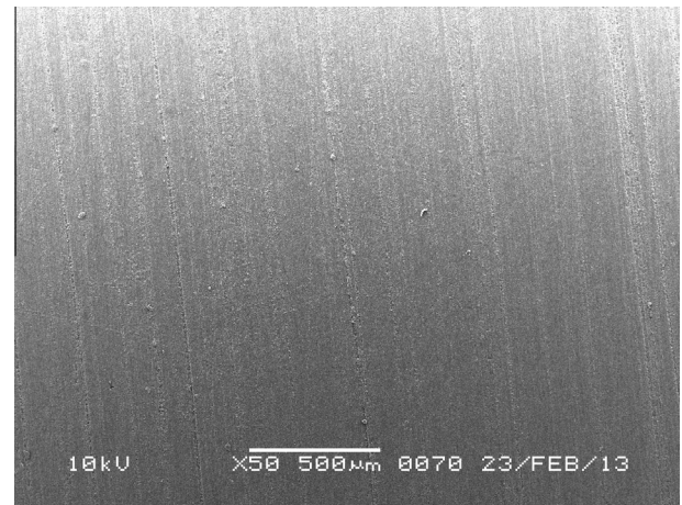
Figure 10 SEM image of visible light cured specimen after polishing using pumice.
