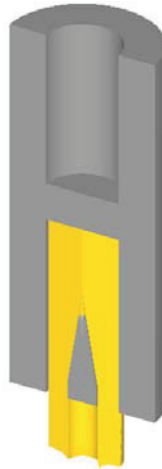
Fig. 1. Schematic illustration of titanium alloy (Ti-6Al-4V) prick hole extrusion
