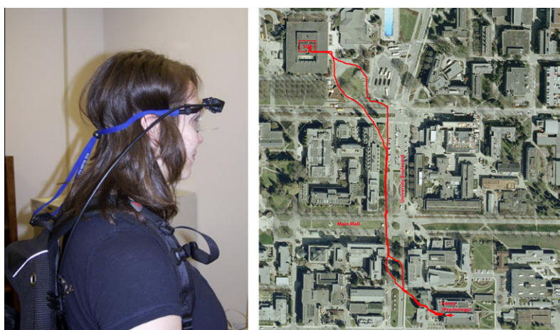
Fig. 1. Left: The ASL MobileEye tracker used to record gaze during walking. Right: The route walked by one participant, as drawn by them on a satellite map of the surrounding campus.
