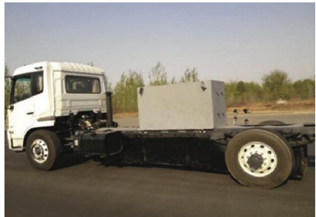
Fig. 4 – The vehicle used for the coast-by test.
