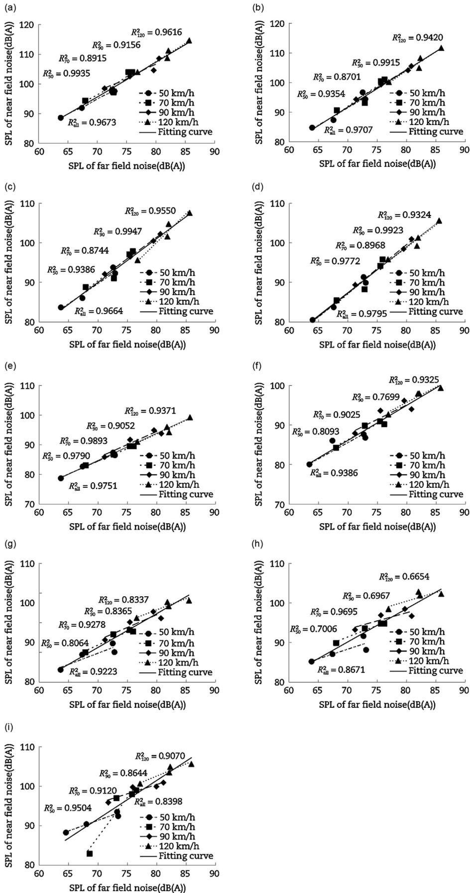
Fig. 6 – Correlation between the near field noise and the far field noise for the 4 sets of tires. (a) 0°. (b) 30°. (c) 45°. (d) 60°. (e) 90°. (f) 120°. (g) 135°. (h) 150°. (i) 180°.
