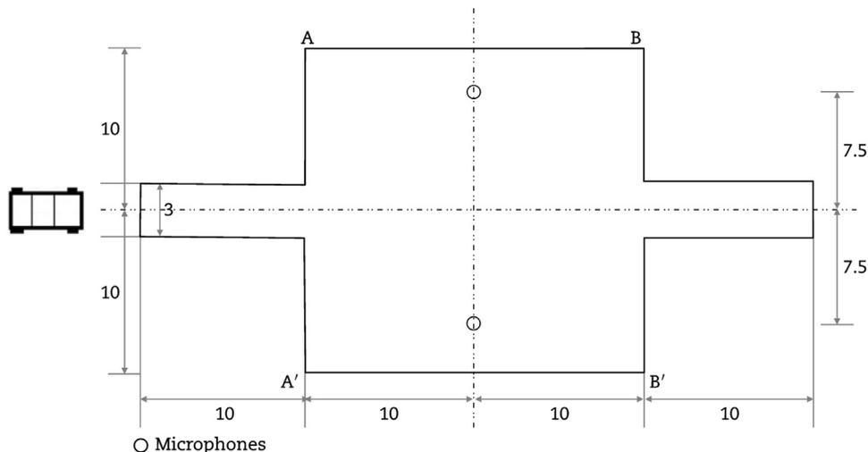
Fig. 5 – The principle diagram of the coast-by method (unit: m).
