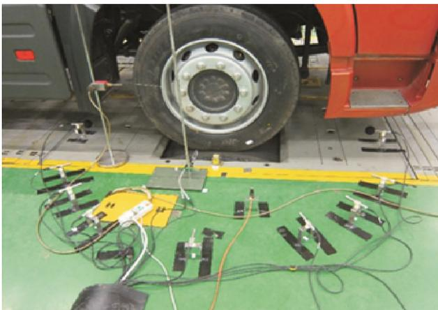
Fig. 2 – Layout of the microphones for measuring the near field noise.
