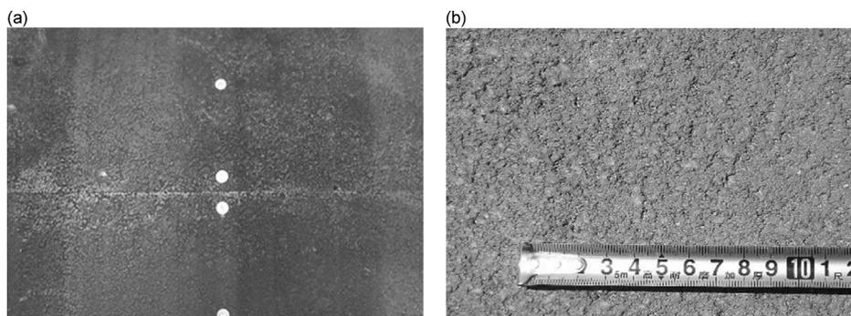
**Fig. 7 – Contrast between the surface of the drum and the surface of the road in accordance with ISO 10844. (a) Surface of the drum. (b) Surface of the road.**
