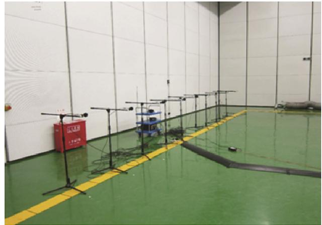
Fig. 3 – Layout of the microphones for measuring the far field noise.
