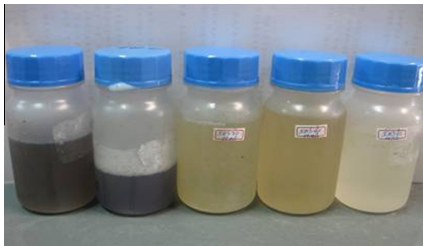
Fig. 7. The change of wastewater color with treatment time of 0, 6, 20, 40, and 60 min (from left to right).
