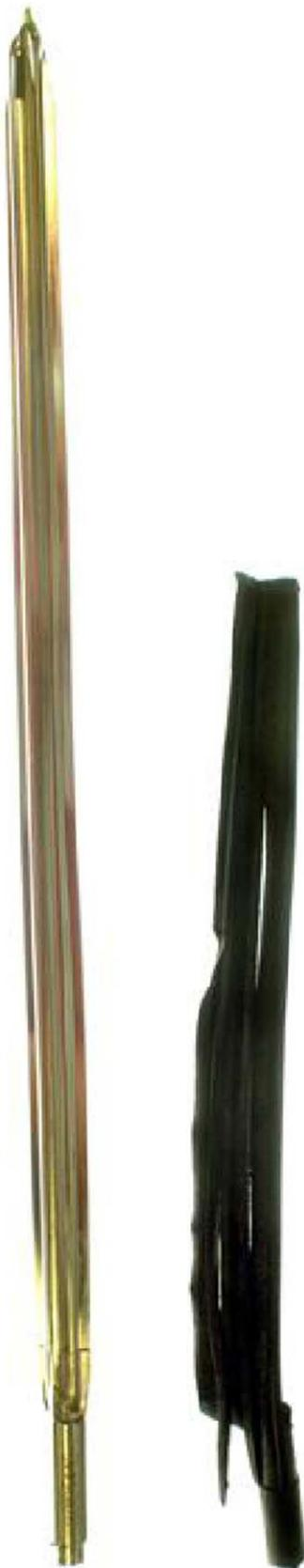
**Figure 1** On the left is an intact Fixion<sup>®</sup> nail inflated and on the right the exploded nail (proximal half) recovered from furnace.
