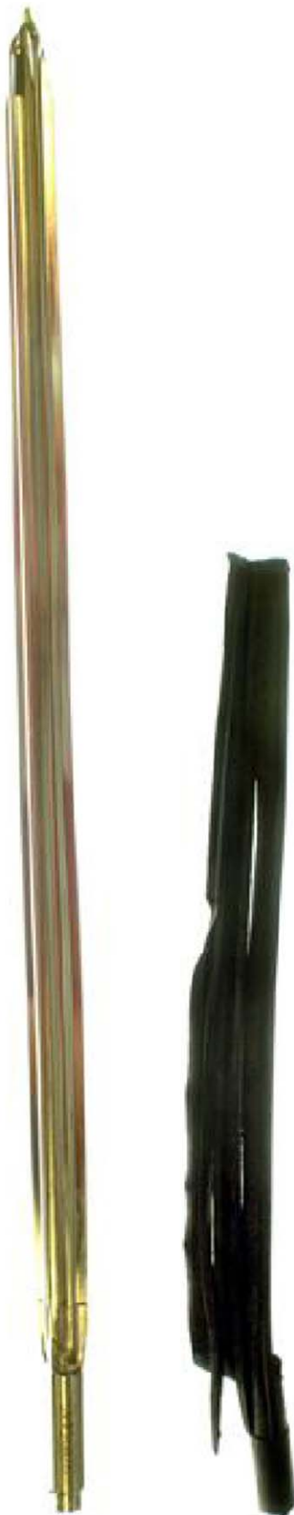
Figure 1 On the left is an intact Fixion ® nail inflated and on the right the exploded nail (proximal half) recovered from furnace.
