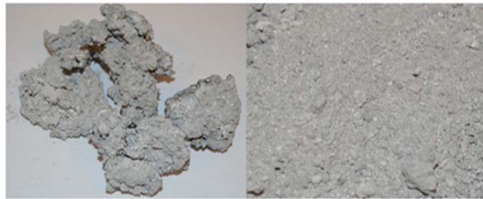
Fig.1. Samples of the white cross aluminum
